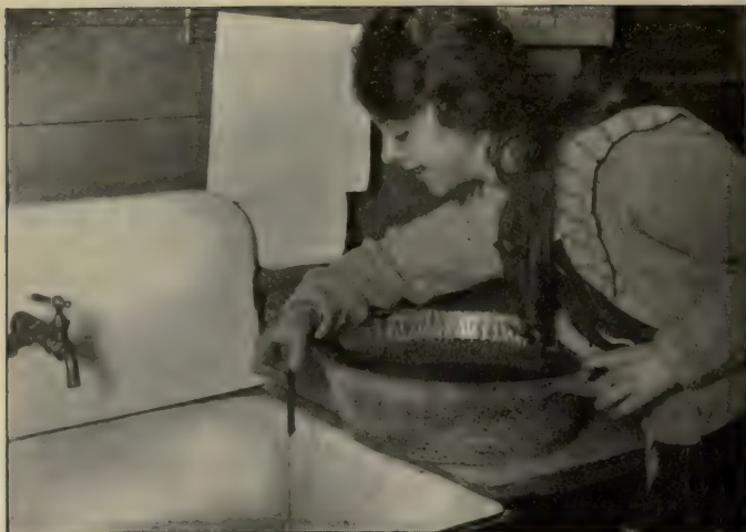
FIG. 8. A siphon. The air pushes the water over the side of the pan.
